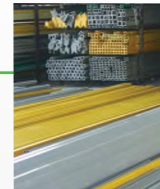
Pultruded FRP profiles are with the constant cross-section structure by a continuous pultrusion process using fiberglass reinforcements with thermosetting resin matrixes. Pre-selected reinforcement materials, such as fiberglass roving, mat, woven fabrics or stitched fabric, are drawn through a resin bath in which all materials are thoroughly impregnated with a liquid thermosetting resin. Typical resins included polyester, vinyl esters and phenolic resin.
